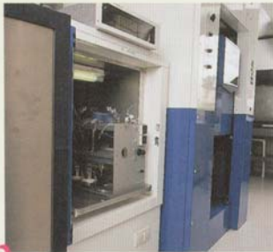
2. Positron emitters are combined in the computerized radiochemistry synthesizer with simple compounds such as glucose to become positron imaging prescriptions.
