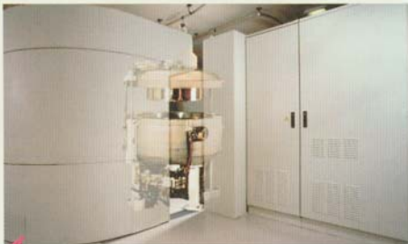
1. The most advanced medical cyclotron – capable of producing positron emitters. 用以生產正電子同位素的最先進醫療迴旋加速器。
